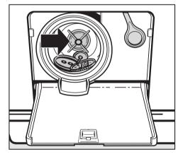
Remove any foreign objects (e.g. buttons, coins, etc) and fluff. Turn the impeller by hand to check that it is free to rotate. Any foreign object causing an obstruction should be reremoved.
